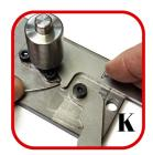
6. Lift the end of the wire over and around the bolt holding Lever #2 [H, I]. Hold the wire flat against the Base, and firmly press Lever #1 against the wire and into the center of the base [J].
