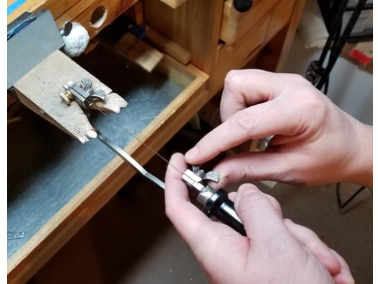
**6. Check the blade tension.** To check the tension of the blade, pluck the blade gently with your thumbnail. When the tension is correct, you'll hear a high-pitched "ping." When it's too loose, you'll hear more of a dull, lower "pong" or "twang." If your blade is too loose, release it from the bottom of the frame and reinsert it, exerting more pressure on the frame.
