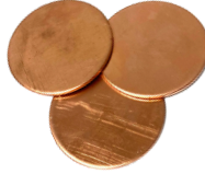
Copper Blanks cut with the FSS (Fast Stamping System)
